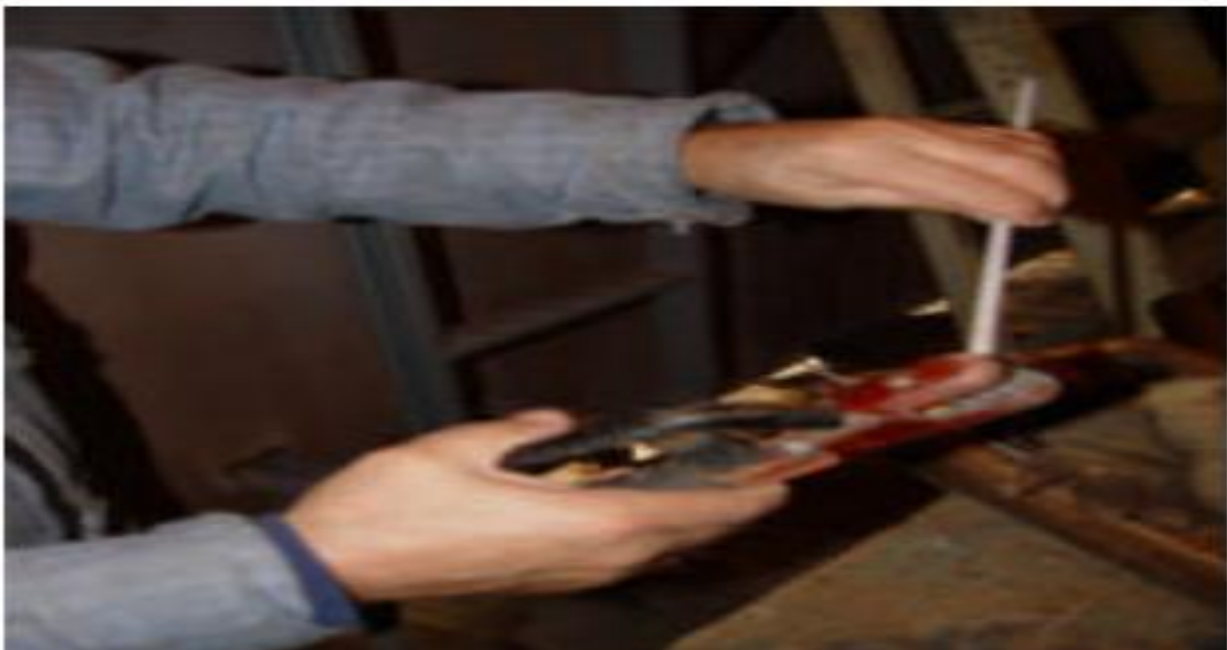
Figure 5: Bare Hands - Requires Dry Insulating Gloves
